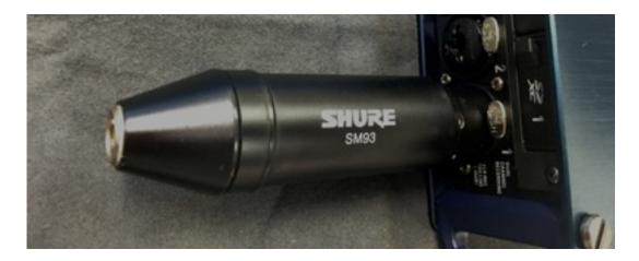
To avoid this issue, insert a microphone cable between the preamp and the F8's XLR jack.
