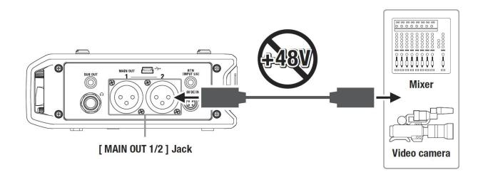
When connecting a video camera or mixer to the MAIN OUT 1/2 jack of the F4, please make sure to turn off any phantom power applied to its input. Since the F4 is not designed to use phantom power, its output circuitry may be damaged.
