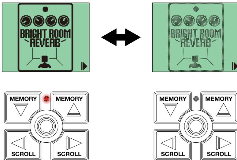
The On/Off indicator lights when the effect is on.
