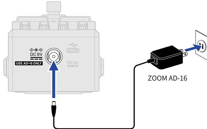
When an AC adapter is connected, the MS-70CDR+ will power on.
