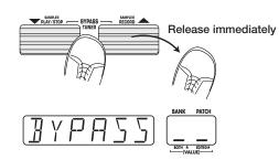
While the GFX-707 is in the bypass condition, the amp simulator is also off and the expression pedal works as a volume pedal.
