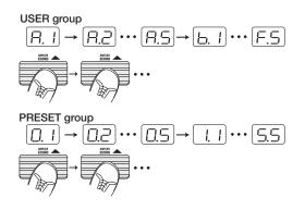
2 To directly switch the bank, use the TYPE (BANK) ▼/▲ keys. This allows you to move to the next lower or next higher bank.
