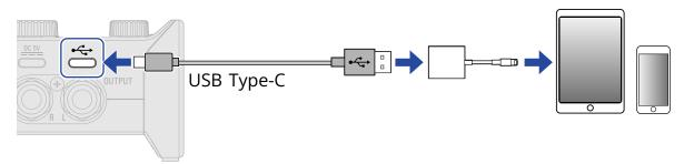
To connect smartphones and tablets, prepare USB cables and adapters that match their connectors as necessary.
