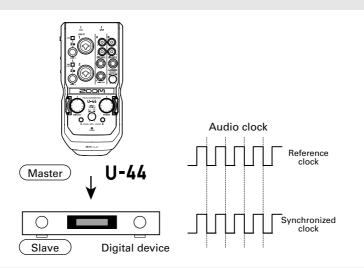
The  $\mathbf{U-44}$  is operating as the master, and the audio clock of the  $\mathbf{U-44}$  and the other digital device are synchronized.
